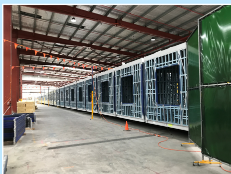
Manufacturing of steel modular cells for integration into the new accommodation blocks.
